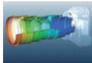
This computer graphic shows a simulation of how much a lens can be deformed by its own weight.
