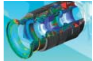
Simulations such as this are used to determine lens damage — where, and to what extent — caused by shock.
