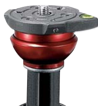
Center column with built-in 50mm half ball locked using the rotating grip located at the bottom of the center column. Tilt range: +15^{\circ}/-15^{\circ} .
