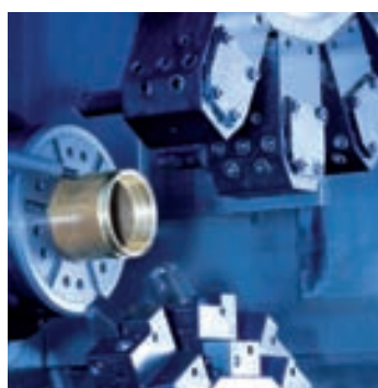
CNC machines turn brass rods into precision rings
