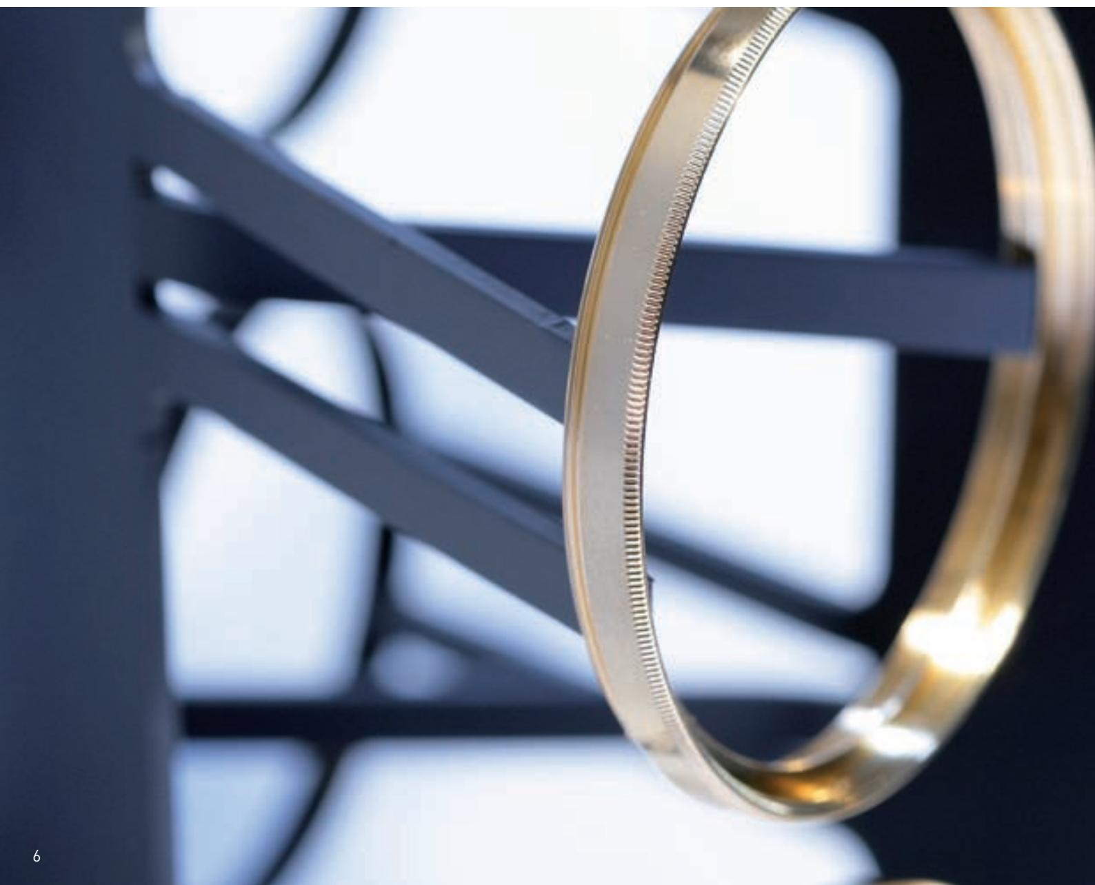
CNC machines turn brass rods into precision rings
