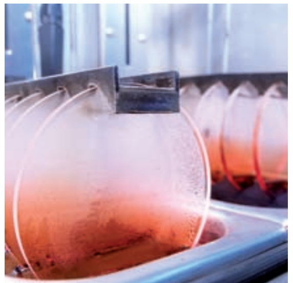
Amplitude-controlled immersion baths – this is how graduated filters are made
